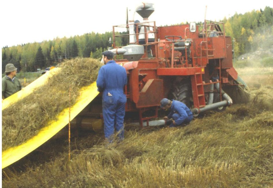
Fig. 2. A modified combine harvester was used to recombine material from straw walkers. Losses from the drum and from the straw walkers were defined in this test. After this test material from sieves was recombined in order to define losses from the sieve unit. Note a bag behind the combine harvester. Material going through the combine was weighted after the test in order to define the mass of the material other than grain. (Photograph: Matti Haverinen).
