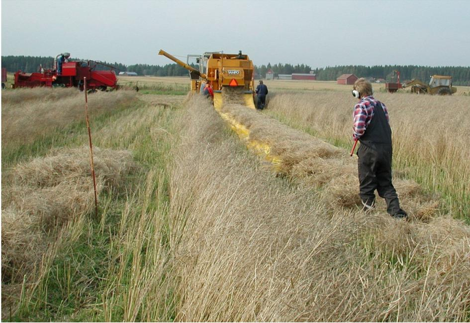
Fig. 1. A combine harvesting test of the spring turnip rape is going on in accordance with ISO 8210 standard. Material from straw walkers was collected on a 25 m long tarpaulin and material from sieves was collected into a bag at the same time (the bag can't be seen because it was coupled to the sieve unit and it was located below the tarpaulin). (Photograph: Lippo Sundberg).
