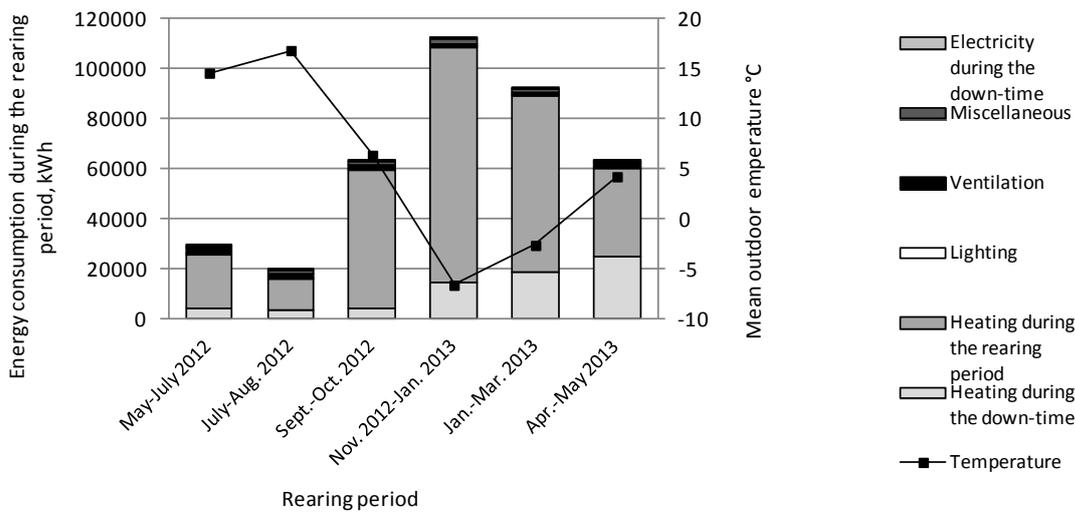
Fig. 10. Mean outdoor temperature during the rearing period and heating energy and electricity consumption during the whole rearing period.
