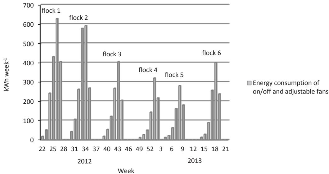
Fig. 6. Weekly electricity consumption of ventilation fans.
