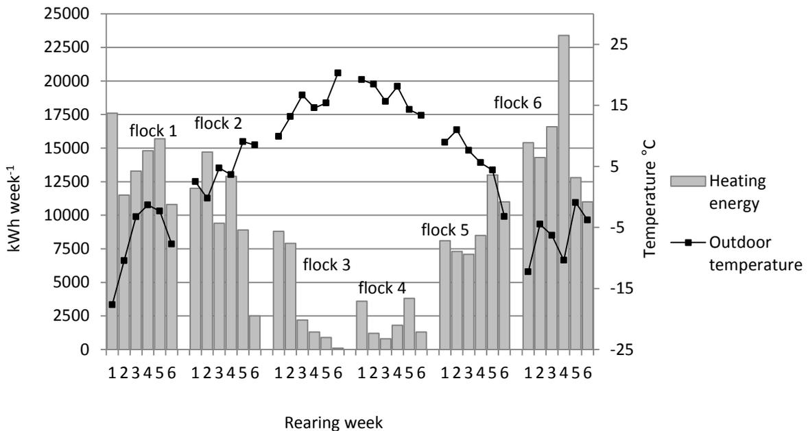
Fig. 9. Weekly average heating energy consumption and ambient temperature during the rearing of six broiler flocks from 30<sup>th</sup> of January 2012 to 7<sup>th</sup> of January 2013. The last rearing week of each flock only includes 3–5 days, depending on the length of the rearing period.
