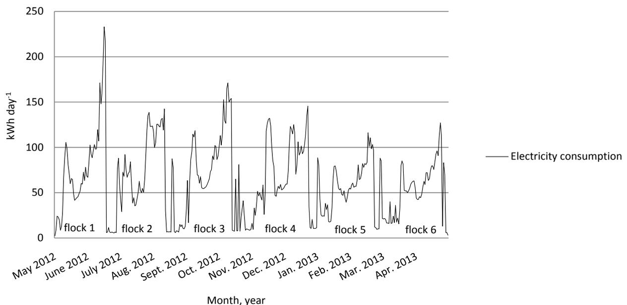
Fig. 5. Daily electricity consumption during the rearing of six broiler flocks.
