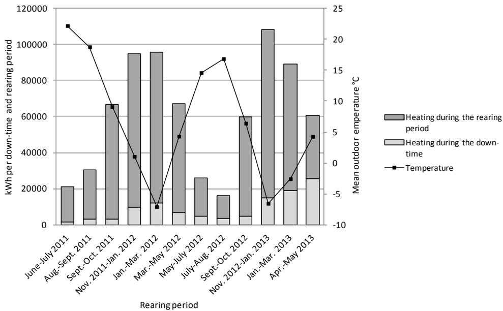
Fig. 8. Heating energy consumption during the rearing of 12 broiler flocks.
