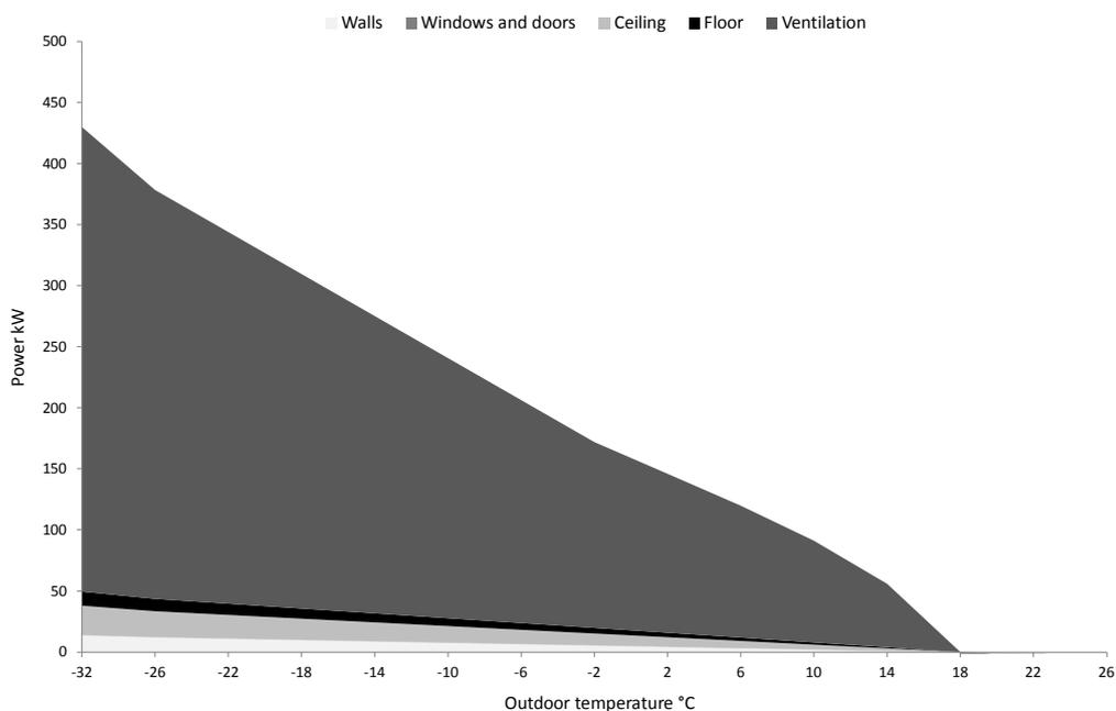
Fig. 3. Example of building heat losses when broiler mass is 1.5 kg.
