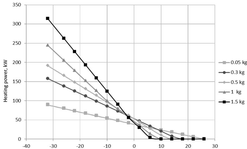
Fig. 2. Example of heating power demand during the rearing period of a broiler flock with different ambient temperatures and broiler weights. 27 000 birds with a density of 17 birds  $m^{-2}$  and with recommended ventilation rates and heat insulation materials (MMM-RMO 2001).
