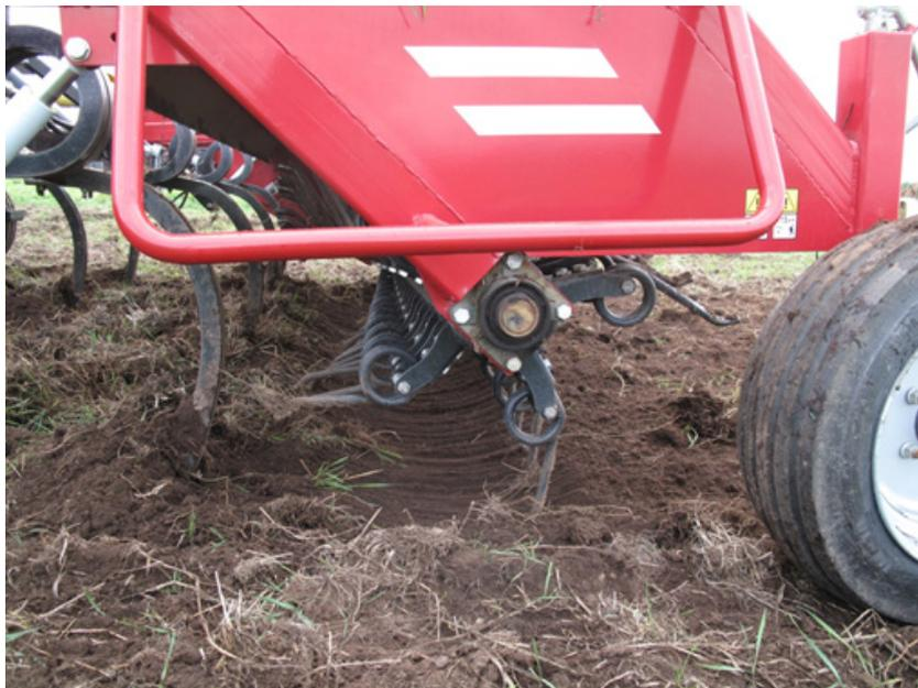
Suppl. Fig. 2. The working principle of Kwick-Finn cultivator: goosefoot tines loosen the soil and after that a PTO-driven rotor throws soil and weed roots into the air.
