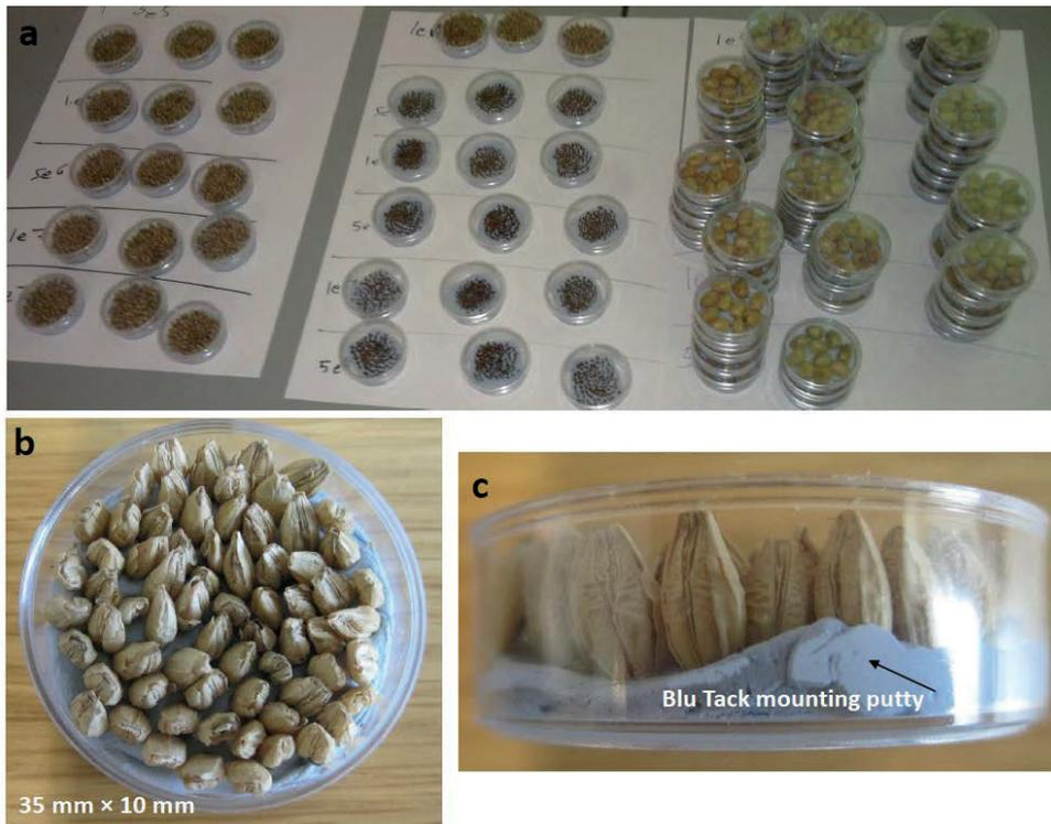
Fig. S1. Dry seed preparation for ion beam irradiation. (a) overview on all three species, (b) view from above and (c) view from side in rye
