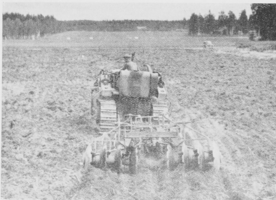
Fig. 7. Reclamation harrowing with a Rome Plow harrow. International TD 14 track-type tractor used as draught machine.
