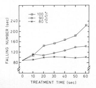
Fig. 1. Influence of hydrothermal treatment at three temperatures on the falling number value of sproutdamaged rye with the initial value of 87. for 60 sec raised the falling number value as much as the treatment for 20 sec at  $100^{\circ}$  C, namely by 55 units. At  $100^{\circ}$  C the treatment for 60 sec raised the value with about 40 units higher than treatment for 50 sec.
