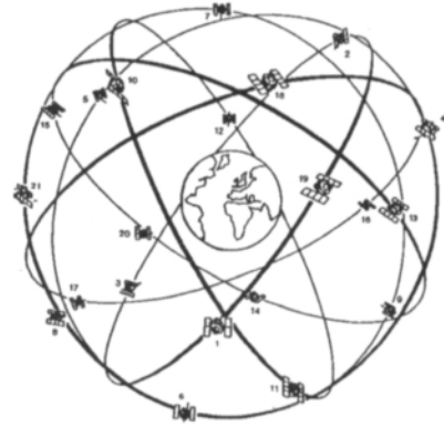
Fig. 65. Orbits of GPS (Global Positioning System) satellites (Sonnenberg 1988).
