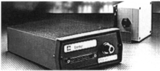
Fig. 75. (a) The DGPS/DR (Differential GPS satellite navigation with DR backup) receiver (front view, size c. 150x50x250 mm) and the DR module and (b) the RTCM-radio beacon (c. 150x75x250 mm). (Courtesy: Trimble Navigation Inc)
