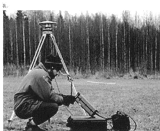
Fig. 74. Tests in 1990–91. (a) The stationary receiver. (b) The vehicle with an installed receiver. GPS antenna shown on the roof. (Photos: Hannu Haapala).
