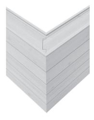
Figure 4. Corner of log walls with a hidden dovetail joint. (Image courtesy of Mammuttikoti) reveal and emphasize the construction technique as well as wall's thickness. Hidden dovetail joint also enables the log courses to be even instead of the traditional half-lapping courses. Thus, when hidden dovetail joint is utilized, log buildings that don't appear as log buildings – by orthodox definition – are created.
