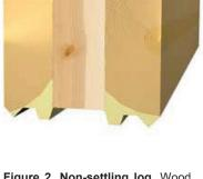
**Figure 2. Non-settling log.** Wood shrinks only in direction perpendicular to grain, and in here the vertical layer of wood in the middle prevents shrinking. (Image courtesy of Matti Alasaarela, Inspis Oy, used with permission)
