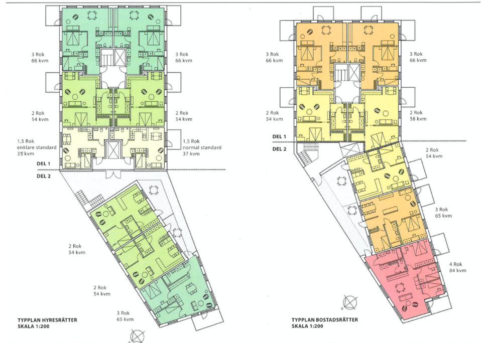
Plan of apartments in rental buildings and illustration of furnished rooms. Source: Tornstaden and T+E Arkitekter.
