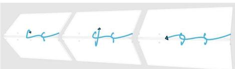
**Figure 8.** (top) Twisted plywood strips clamped at their short edges before connected by lacing technique, (bottom) “Clove Hitch End” lacing/knot technique.
