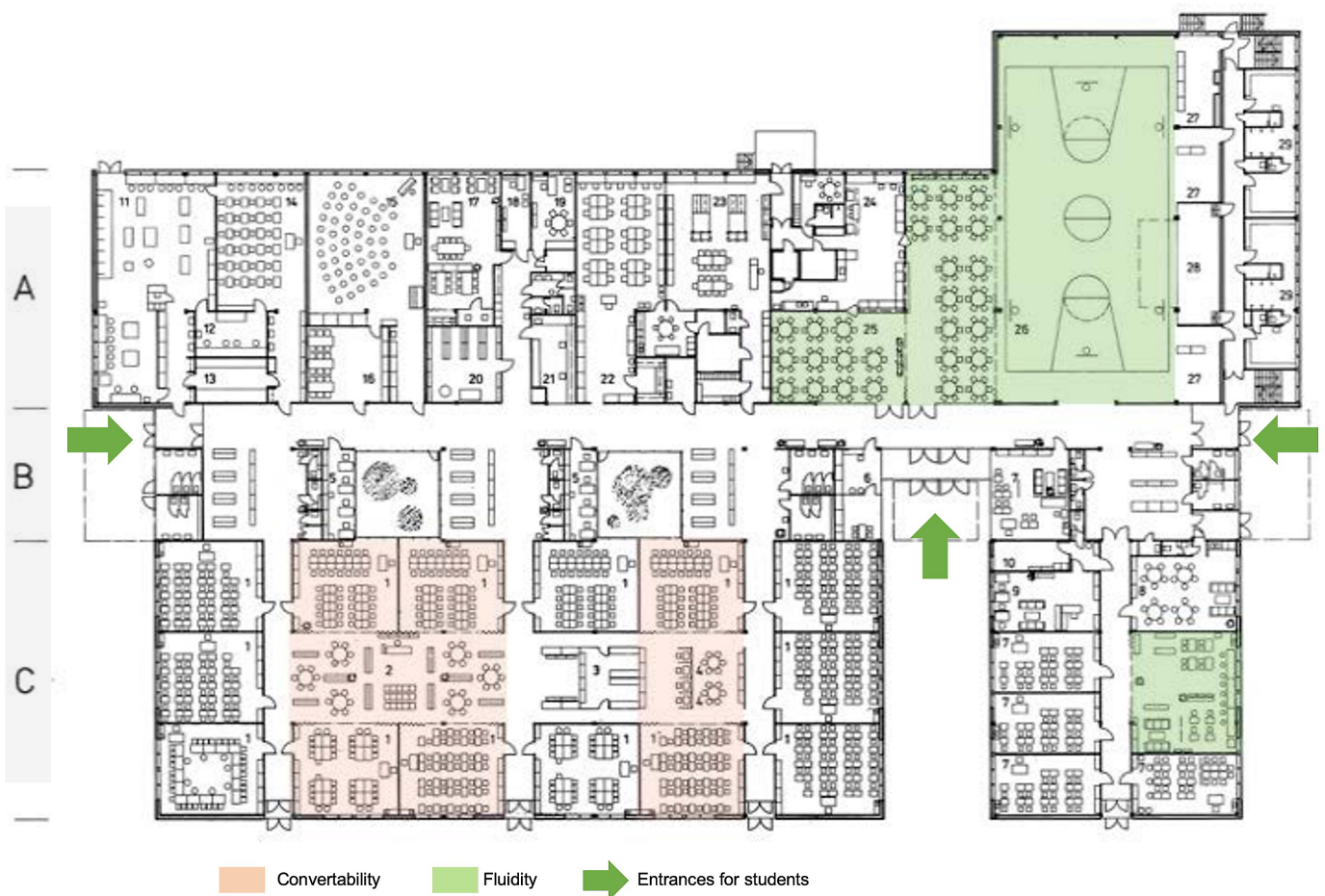
Figure 2. Convertability and fluidity of the learning spaces in Myllyhaka school. The plan is not in scale.
