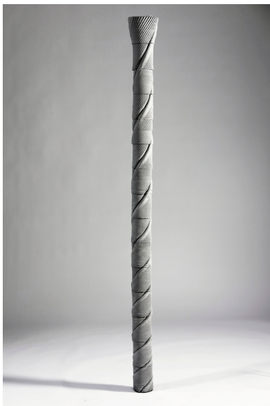
Prototype for a 3D printed ceramic cladding system as a practice-based research project design to consider the application of clay as a protective and decorative cladding material for structural steel
