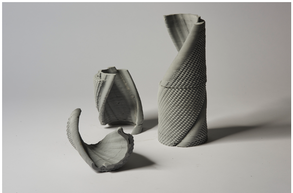
Figure 2. Woven textile expression on the surface of the tiles. This effect is generated by how the print path extrudes the soft clay and how the layers of material interact with each other.
