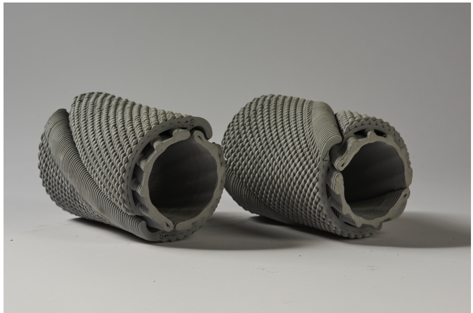
Figure 3. Seams, fold and knots. The connections at the scale of material junction up to the scale of how the pieces interlock are all based on textile conventions translated into 3D printed clay
