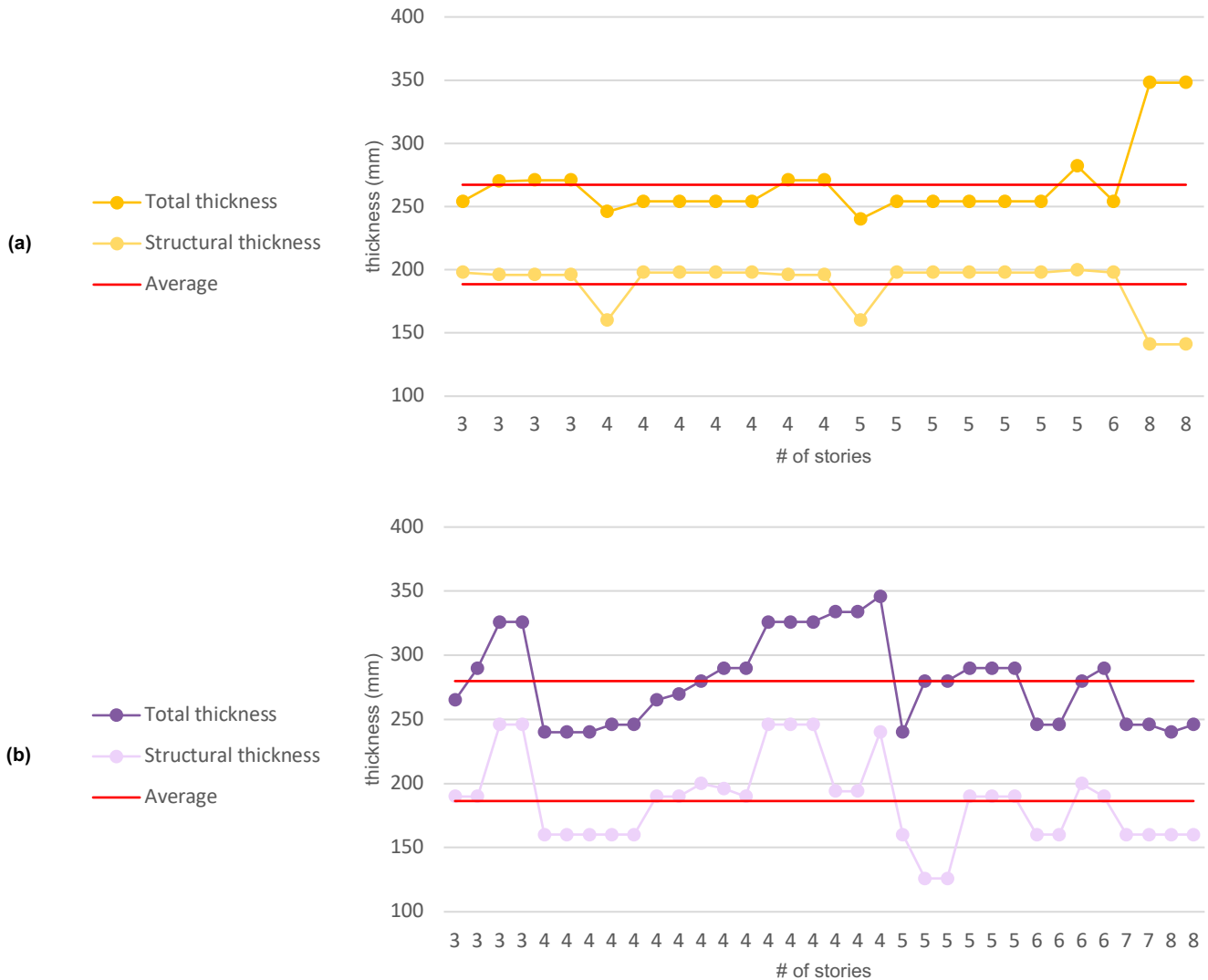
Figure 17. The structural thickness and total thickness of party walls based on the number of stories in (a) 2D panel construction method; (b) 3D volumetric construction method.
