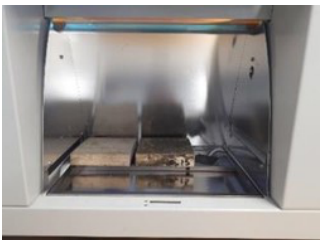
Figure 9. Suntest CPS+ device - suntest with two formwork wood samples
