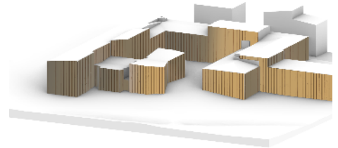
Figure 21. Aalto Civil Engineering Building: South-East View predicted color gradient-after being exposed to one month outside
