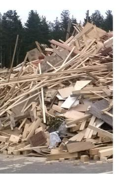
Figure 2. Demolished wood in an ordinary sorting facility: inconsistent in quantity, quality, dimensions, availability and compatibility. Photo courtesy of Paavo Huuhka.
