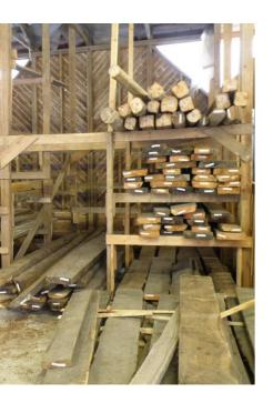
Figure 3. Deconstructed wood in a salvage yard: organized based on length and component type, but still varying in many respects.
