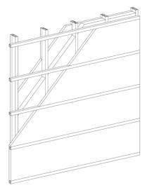
Figure 4. Distribute functions for different structural members. A wall structure with high U-value (0.17) made of thin studs: two-byfours bear loads, inner and outer battening provide space for thermal insulation.
