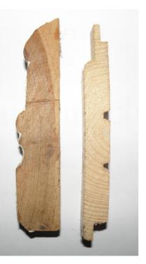
Figure 7. Cross-sections of an antique trim (left) and a modern panel (right). The former is extremely dense, almost entirely made of durable heartwood and the heartwood is towards the exposed surface. The latter is coarse-grained and has no heartwood.
