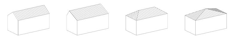
Number of different joist lengths increases
