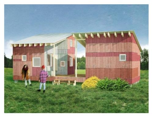
Figure 21. Define ranges instead of fixed properties. A facade cladding with ranges of red and grey colours; the window layout can also tolerate windows of varying dimensions (design and image by Szymon Galecki).
