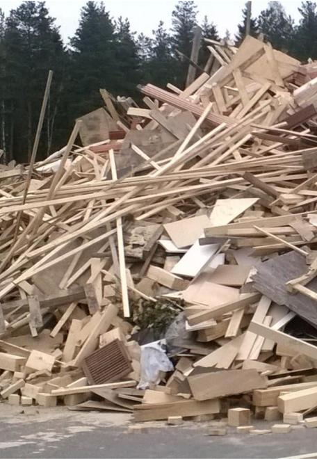
**Figure 2. Demolished wood in an ordinary sorting facility:** inconsistent in quantity, quality, dimensions, availability and compatibility. Photo courtesy of Paavo Huuhka.
