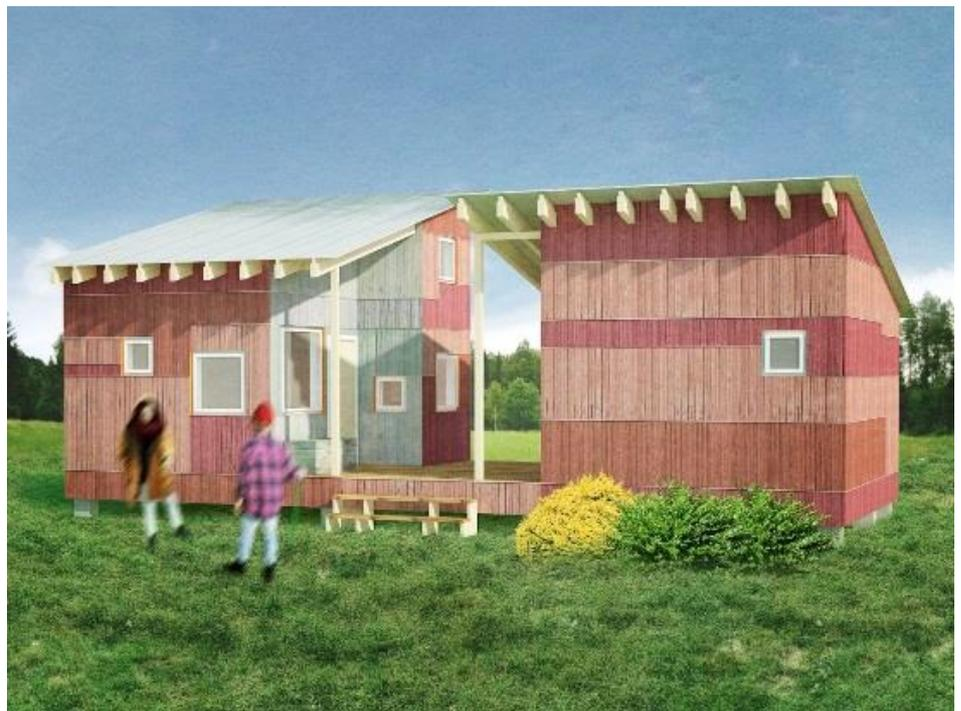
**Figure 21. Define ranges instead of fixed properties.** A facade cladding with ranges of red and grey colours; the window layout can also tolerate windows of varying dimensions (design and image by Szymon Galecki).
