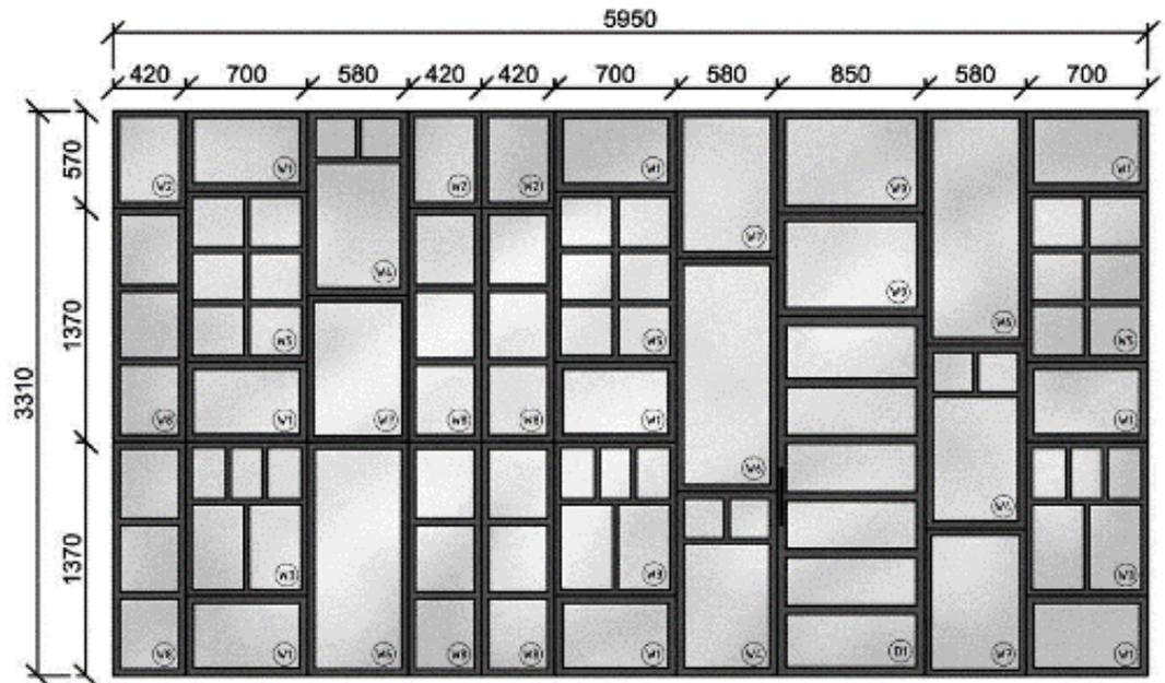
**Figure 24. Combine creatively.** A schema for a glass wall made of salvaged windows (design and image by Michala Konarikova).
