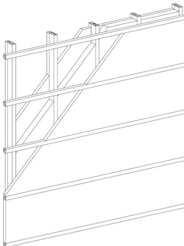
**Figure 4. Distribute functions for different structural members.** A wall structure with high U-value (0.17) made of thin studs: two-by-fours bear loads, inner and outer battening provide space for thermal insulation.
