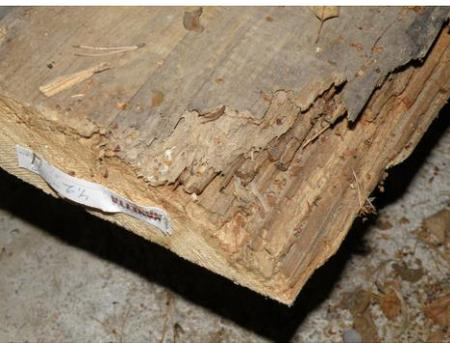
**Figure 8.** Rot at the end of a salvaged floorboard. Damage in wood is easy to recognize visually.
