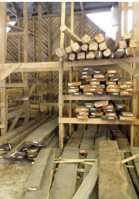
**Figure 3. Deconstructed wood in a salvage yard:** organized based on length and component type, but still varying in many respects.
