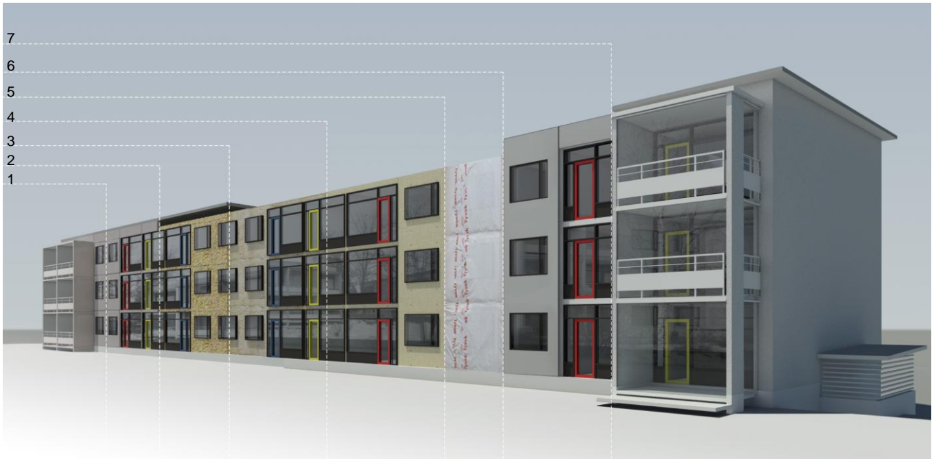
Figure 5. The TES EnergyFacade retrofit process of Case A visualized. Stages from the left: 1) original building, 2) removal of old balconies, the external layer of concrete and old thermal insulation (old windows are still intact for weather protection), 3) the assembly of soft thermal insulation as adaption layer, 4) the assembly of an airtight layer, 5) the assembly of vertical, pre-fabricated, timber-based new facade elements including new passive house standard windows and the removal of old windows beneath, 6) finalization of the renewed facade with a new roof and detailing, 7) the assembly of new balconies. Image by Ville Riikonen, Aalto University.
