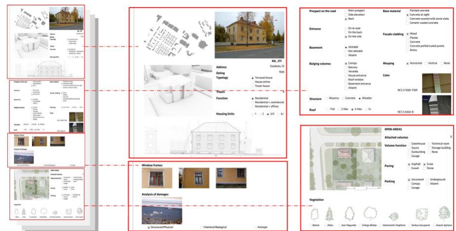
Figure 16. Example of digital inventory for the description of buildings in Raksila. The record card includes all the information collected on field through the survey, CAD drawings, 3D modelling, investigation on site and historical info.
