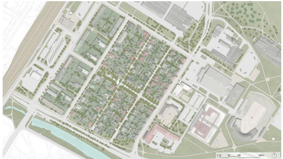
Figure 2. The map of Raksila updated on the base of the point cloud from the digital laser scanning survey. The map includes all different levels of information, from the measures to the characteristics of buildings, streets and vegetation.
