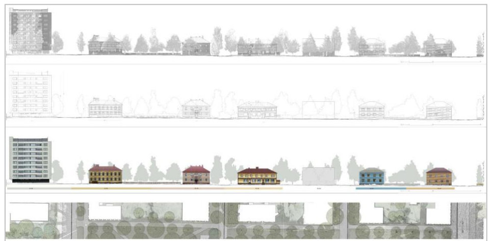
Figure 15. Description of one street front of Raksila neighbourhood. CAD drawings allow the check of measurements. Photomaps define the real image of the place and give information on colours. The map redrawn from the point cloud has been enriched with the description of the green system of trees, paths and roads with identification of different materials.
