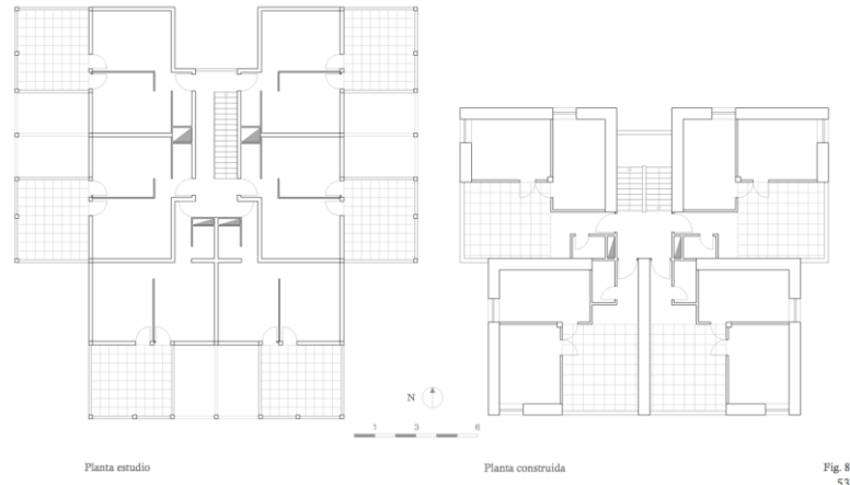
Figure 14. The 'Tower': ATBAT Group theoretical design (left) Bodiansky built project (right). Author's drawing, 2018.
