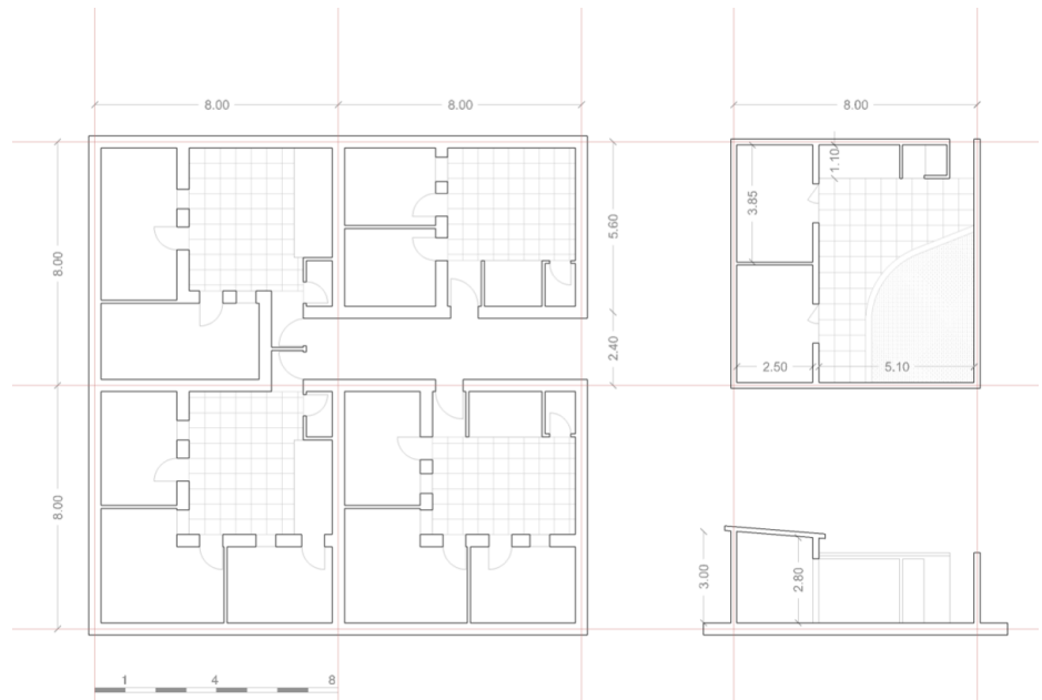
Figure 7. Écochard Grid: 8x8 m Four-patio-house cluster. Author’s drawing, 2018.
