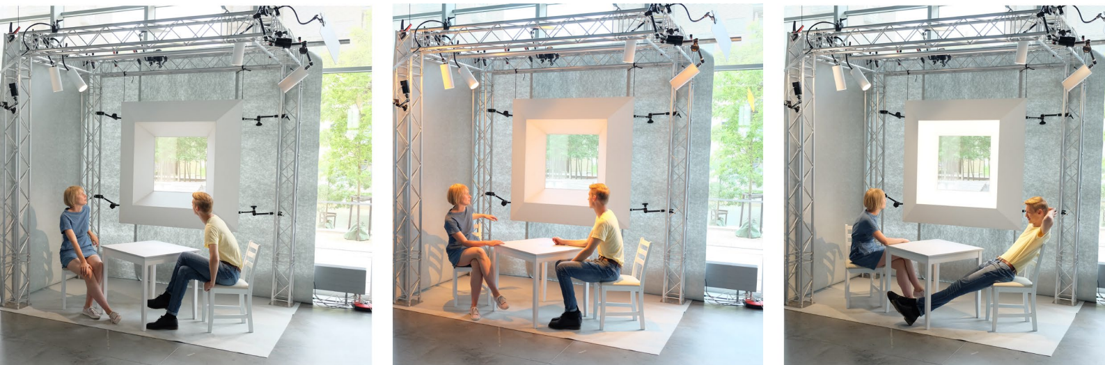
Figure 3. Three states of the adaptive lighting in a situation with two participants. This is staged for the camera and therefore the changes are made very explicit. In the ambient settings of adaptive lighting only nuances appear.
