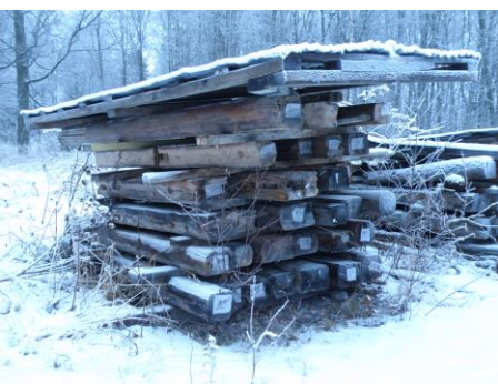
Figure 12. Reduction of length. Very few of the logs stored in this salvage yard span more than 2 m.
