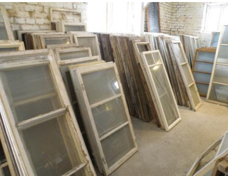
Figure 14. Lack of standardization. None of these windows are exactly the same.
