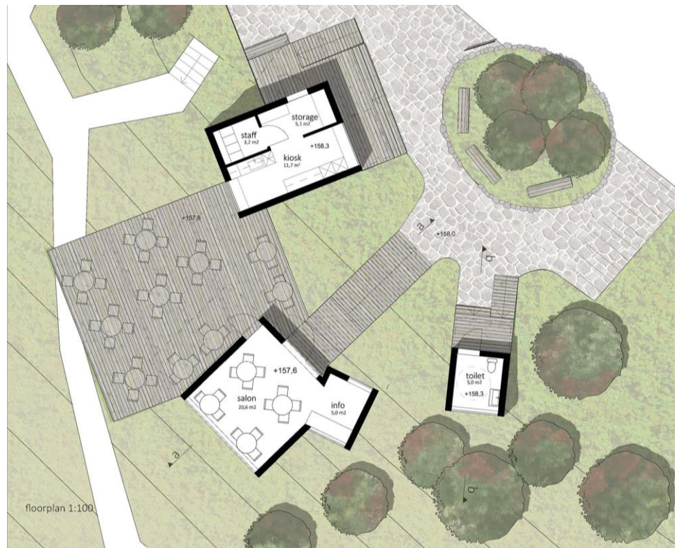
Figure 16. Divide the spatial program into smaller units. The plan of this café pavilion consists of multiple freestanding volumes (design and image by Paula Tiainen).
