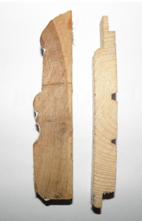
Figure 7. Cross-sections of an antique trim (left) and a modern panel (right). The former is extremely dense, almost entirely made of durable heartwood and the heartwood is towards the exposed surface. The latter is coarse-grained and has no heartwood.
