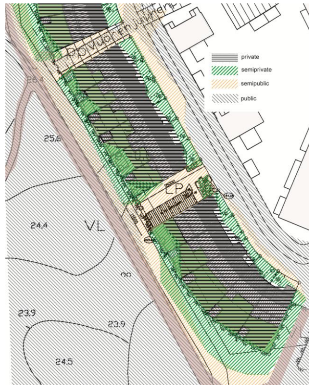
Figure 12. Vuorenjuuri spatial hierarchy: the residential experience. The interpretation is the author's, based on the residents' interviews and reflection to previous material, including Hansarinne.
