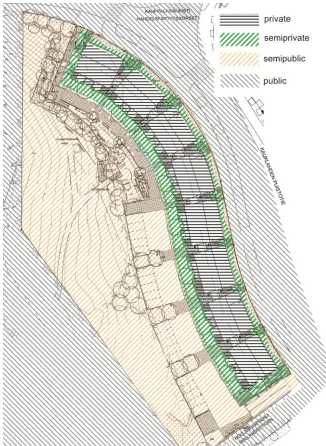
Figure 6. Hansarinne spatial hierarchy: the planning approach. The interpretation is the author's, based on the planning understanding.
