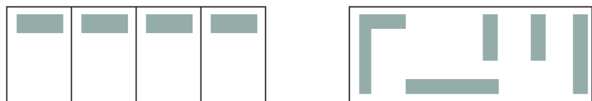
Figure 1. On the left the benches are located in separate rooms, and in comparison, on the right benches are located in the same room. Locating benches in the same space allows more various organizations of laboratory furniture and enables, for example, shared use of instrument maintenance. (Yläoutinen et al. 2014)
