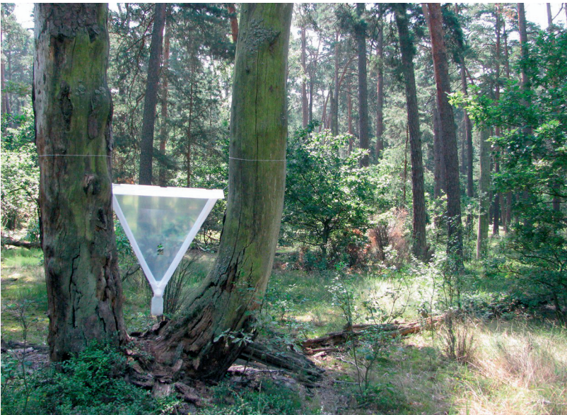
Fig. 2. An IBL-2 type screen trap used to catch insects in Kampinoski National Park.
