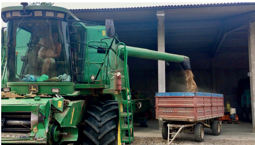
Figure 7. The combine harvester shoots out winnowed wheat berries into a trailer for drying. Photo credit: Author.
