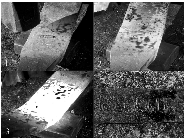
Fig. 8. Attaching of inlays with the optimal method: 1. cold rod placed on the surface of the hot blade blank, 2. rod is hammered to make it sink completely into the blade, 3. after all inlays on one side are sunk, they are welded in a high temperature, 4. detail of welded inlays on a blade blank. Photographs: Mikko Moilanen.
