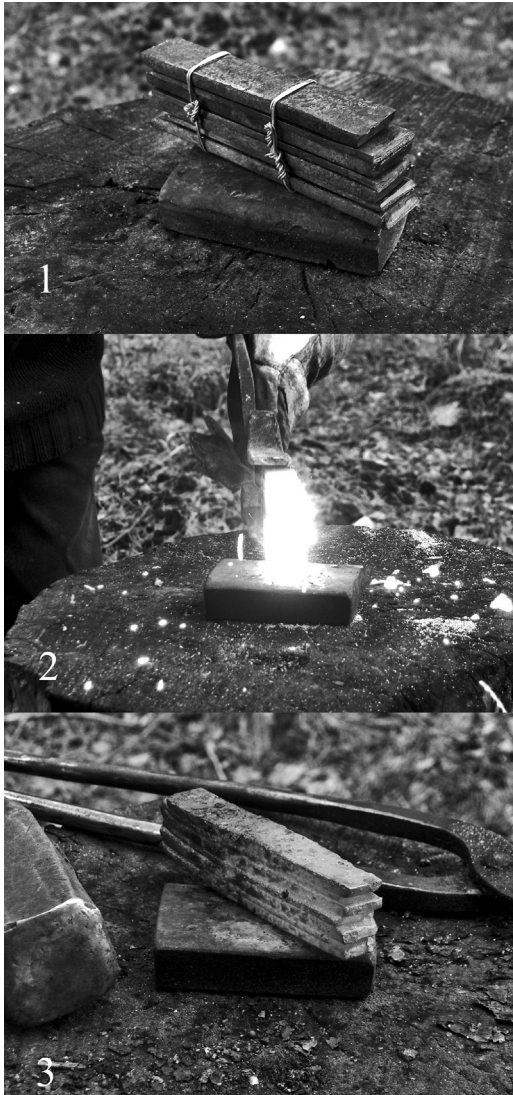
Fig. 6. The making of a pattern-welded pack: 1. a pack made from alternating sheets of iron and steel, bound together with iron wire, 2. forge-welding the pack by hammering, 3. completely welded and solid pack. Photographs: Mikko Moilanen.
