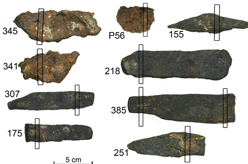
Fig. 2. Metallographically studied blooms, billets and iron bars. Rectangles mark the location of the cut cross-section. Illustration: R. Saage.
