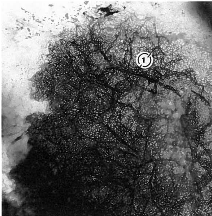
Fig. 8. Photomicrograph of a quenching microfracture in quartz, waste piles of the Kopinkallio quarry. The fracture is partly filled with organic tissue material (1). These fractures give the typically mottled, dark brown appearance to the ancient and long-buried heat-treated quartz (see Fig. 3). Transmitted light. The picture area is 0.78 x 0.78 mm.
