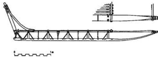
Fig. 22. Two-legged central-grooved "seal-hunting sledge".
