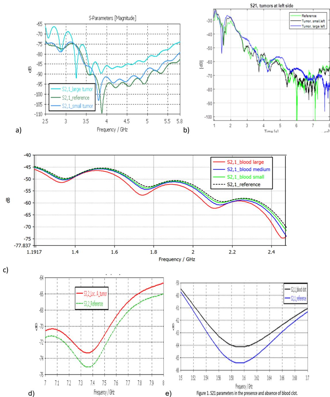
Figure 1. S21 parameters in the presence and absence of blood clot.
