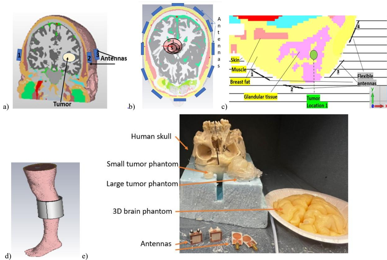
**Figure 2.** The simulation models used in the studies for detection of abnormalities in the brain (a-b), breast cancer (c), blood clot in the leg. The measurement setup with real a human skull and 3D realistic shaped brain phantom prepared for brain tumor studies (d).
