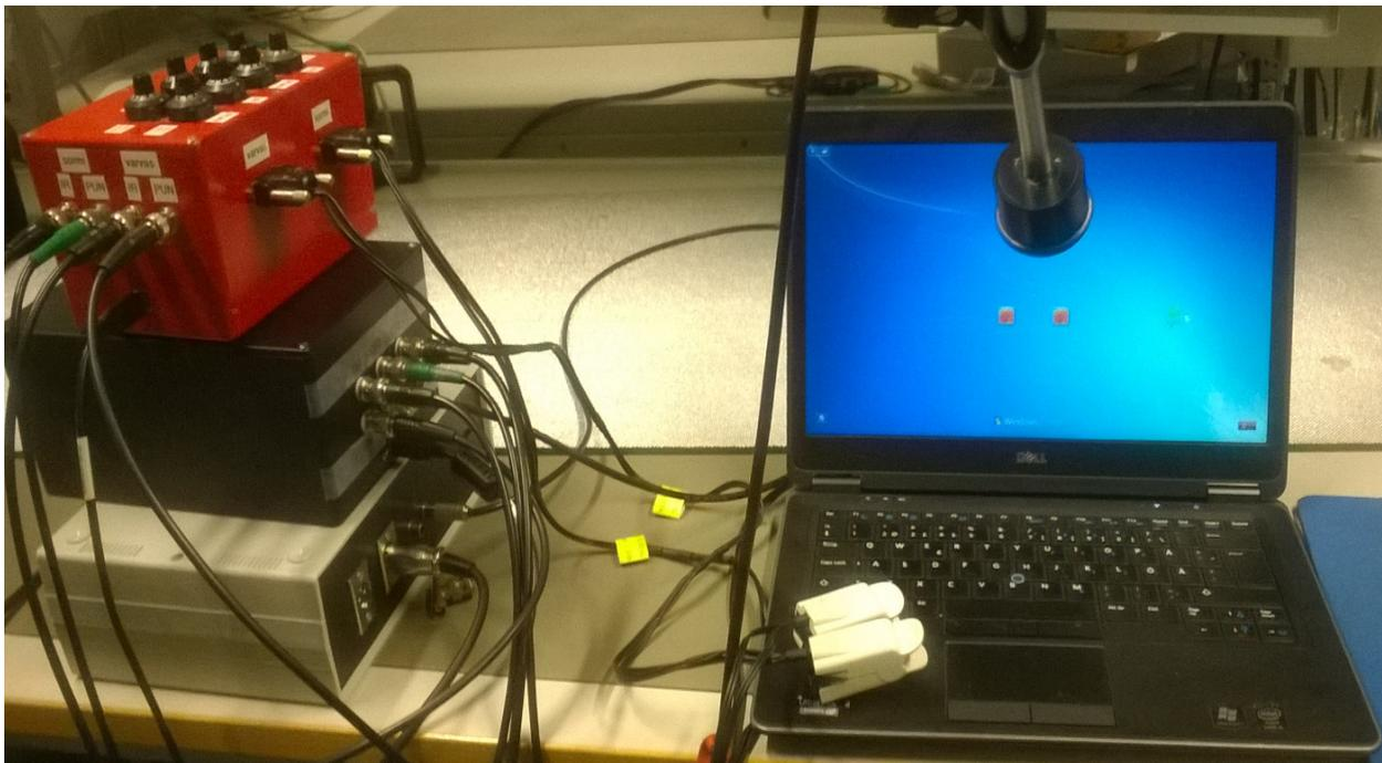
**Figure 1.** Phase sensitive detection (PSD) block schematic (top), the PPG device on the top and the measurement box (bottom).
