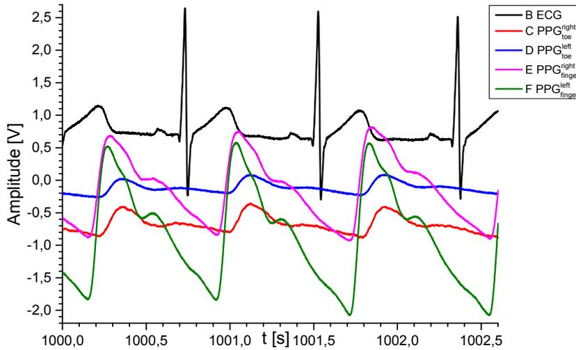
**Figure 2.** The measured ECG (black), and PPG pulse waves from right (magenta), left (olive) index fingers, right (red), and left (blue) second toes.
