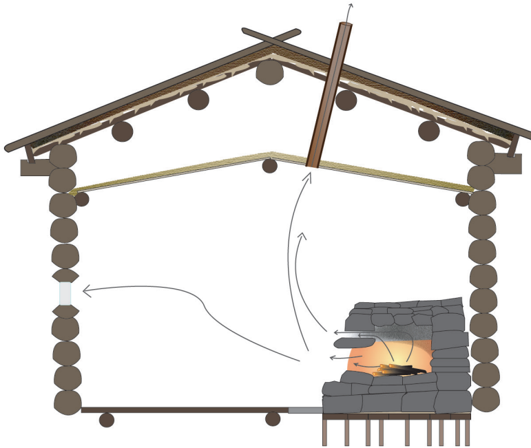
Fig. 5. Appearance of the ceiling did not necessarily succeed the innovation of chimneys and flues, but the progress could have been the opposite. A drawing presents a smoke cabin, where the smoke has directed outside through a wooden pipe. Ceilings reduced the space to be heated and thus saved firewood and time needed for heating. Furthermore, they provided extra insulation and an upper floor for storage. Drawing: Liisa Seppänen
