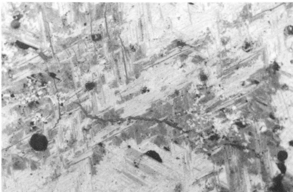
Fig. 15. Widmanstätten structure of copper matte.  $\times 200$ .
