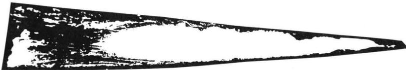
Fig. 7. Laminations of iron on the back of a steel-cored knife from medieval Goltho, UK.  $\times 7$ .
