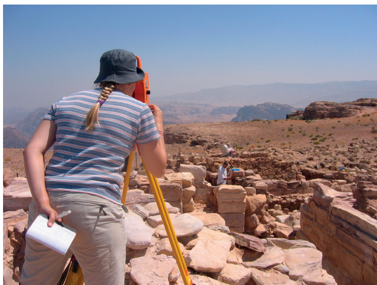
Figure 11. Anna Annila operating the total station at the site, Rikhard Holmgren is holding the prism in the background (2007 field season). Photo: Antti Lahelma.
