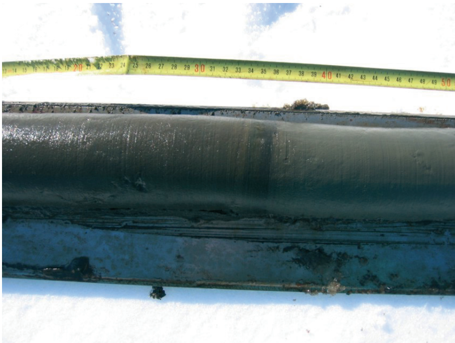
Fig. 14. The sediment sequence at 175–210 cm. At the bottom (on the right) light greenish grey clay gyttja from the Baltic Sea, at the top dark brown gyttja from the isolated lake. (Photo: A. Miettinen 2005)
