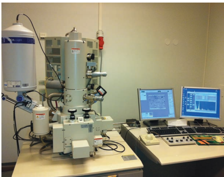
Figure 3. The FESEM-EDS (Hitachi S-4800 with an Oxford Instruments 350 INCA energy-dispersive X-ray microanalysis system) instrument, based at the Department of Inorganic Chemistry at the University of Helsinki, employed in the archaeometric studies discussed in this paper. Photo: E. Holmqvist.
