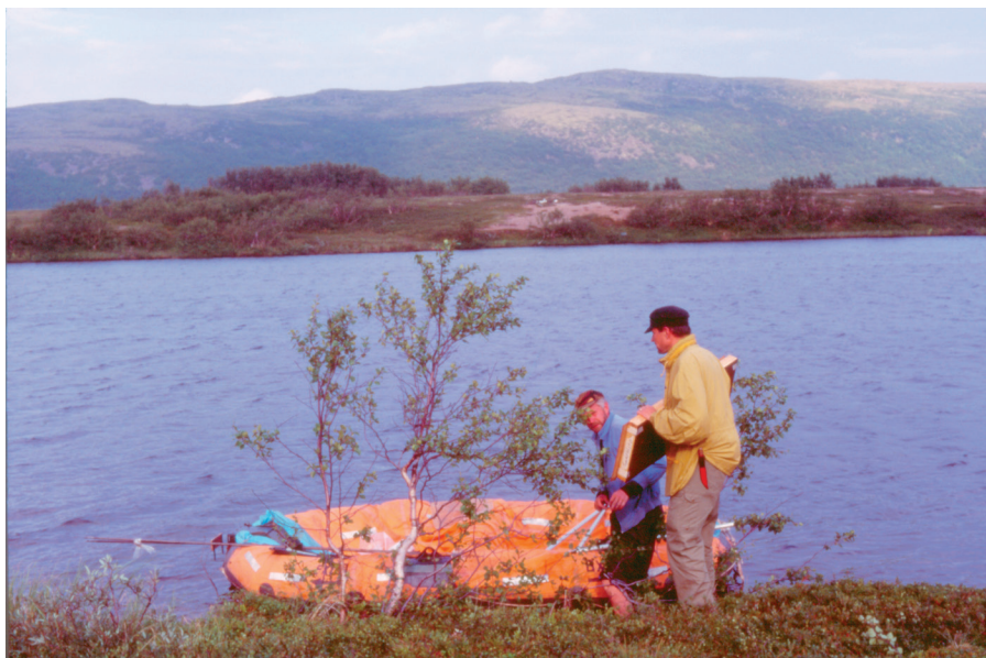
Figure A1.8. The rubber boat used in coring operations was anchored by a rope from shore to shore. The piston rod of the corer was anchored in the device on the left end of the boat. Looking towards the east across Lake Sol-datskoye. Photo: Matti Saarnisto.
