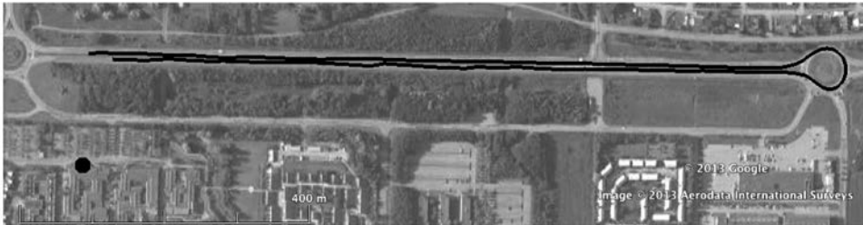
Figure 1. Trajectory from kinematic experiment. The master receiver is marked with a black dot in the lower left corner.
