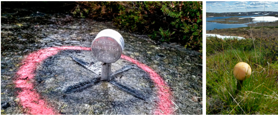
Figures 3a-b. Norwegian boundary marks. Photographs by Leiv Bjarte Mjøs. Figure 3a. Chiselled cross in rock renewed with standard aluminium boundary mark was first introduced in 1980.
