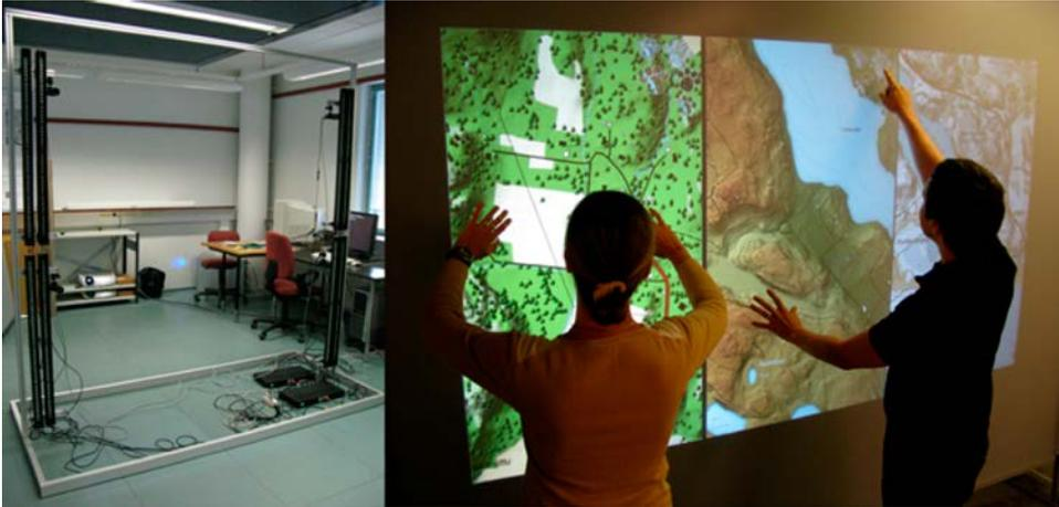
*Figure 2. Our original rear projection setup for the multi-touch system, with a projector, computer, IR cameras and IR lights at the back (on the left) and a large canvas on the front displaying the map application (on the right).*
