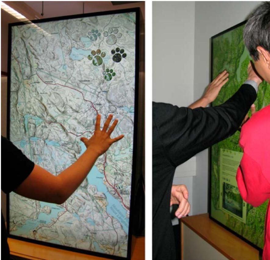
**Figure 3.** A single Multi-touch Cell Advanced display showing our MenoMaps Tassu map application. The 'Topographic Map' on the left and the 'Forest Map' on the right.
