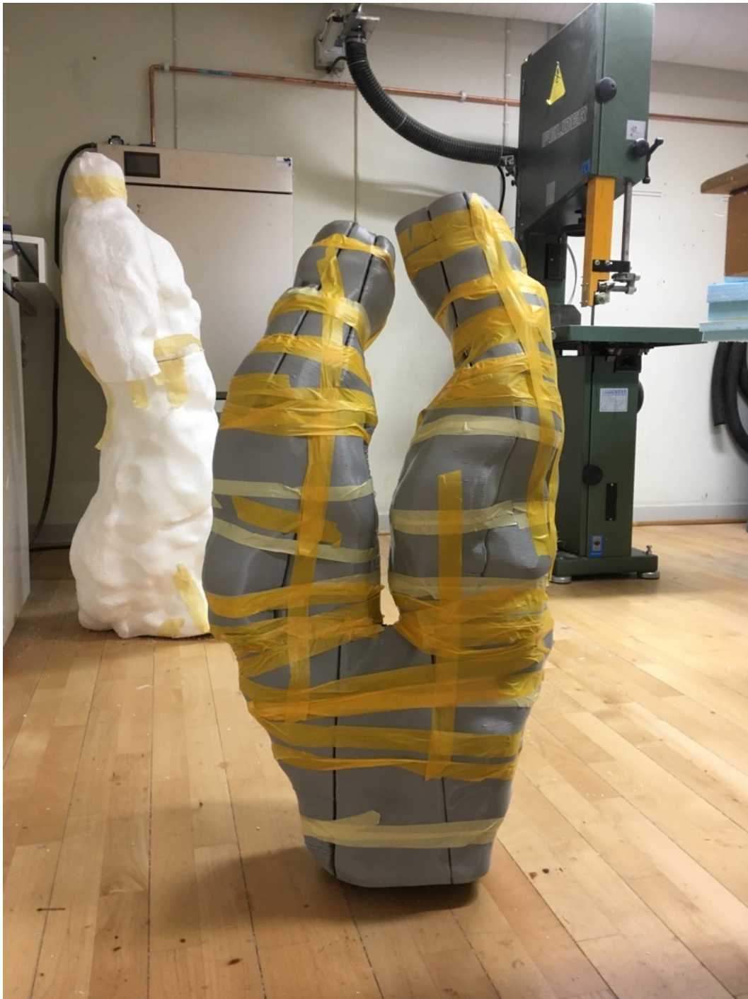
Figure 9. The Sediment Trouser mould was 3D printed using bioplastic. It was printed in parts to facilitate removal from the shrunken textile-form.
