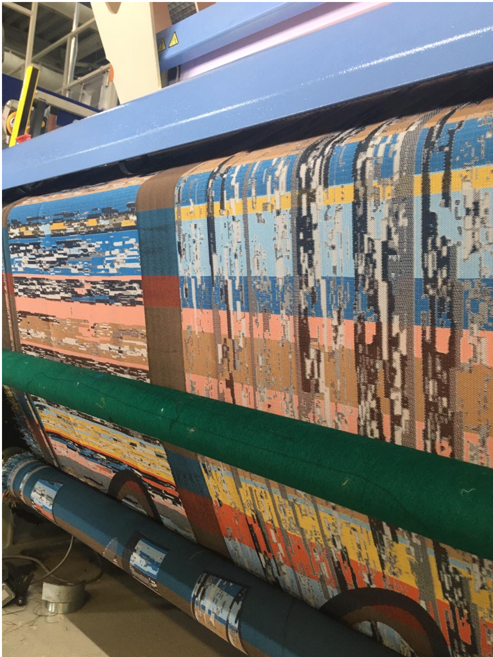
Figure 8. Three variations of the Sediment Trouser woven across the width of the loom. After failing in the initial tunic, the seams for the remaining garments were widened and the bindings changed. The crotch seam (at bottom) affects the surface pattern, an example of the impact of multimorphic design practice.
