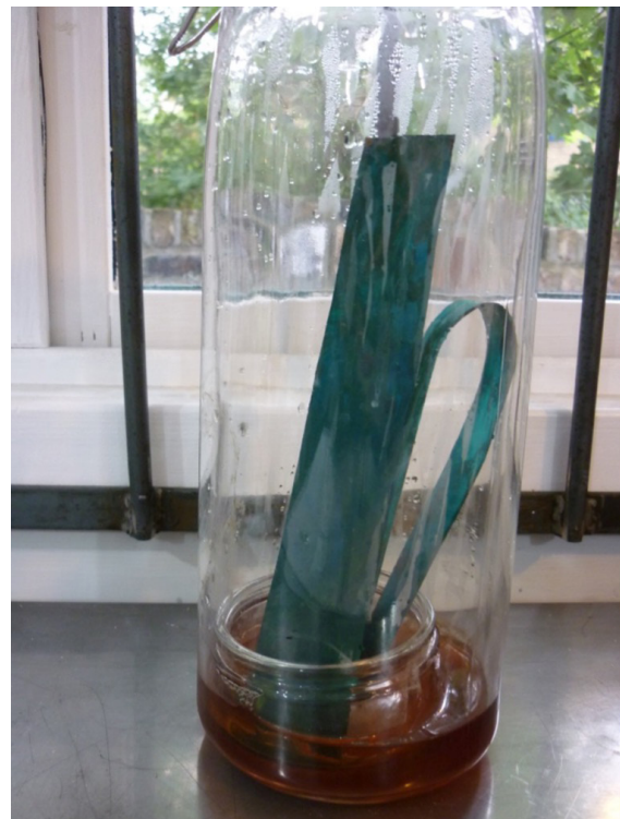
Figure 5 Copper suspended over vinegar in a sealed container to create verdigris. The verdigris pigment is applied over Naples Yellow to achieve the green of the Magdalen's dress seen in Figure 4. Photo: R. Whitman
