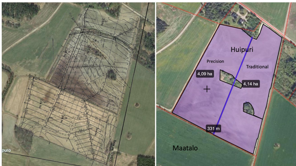
Fig. 1. Test Plots. On the left, a drainage map; on the right, the division of the Huipuri field for precision farming and traditional cultivation methods. The Maatalo plot was a test area where the functionality of the technology was evaluated.
