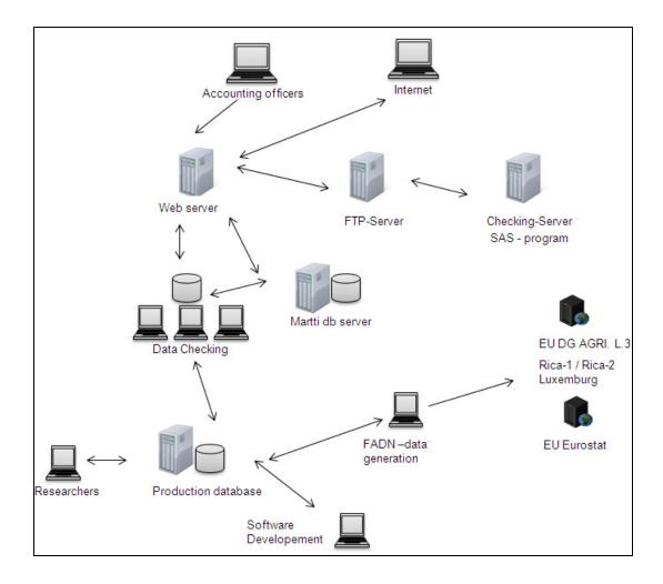
Fig 1. An overview of the web application system used as data system in Finnish profitability bookkeeping.
