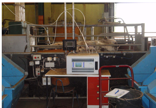
Figure 2. A two-point F10 Multi-gas analyzer set-up in operation with a cow in feeding kiosk getting her concentrate supplement while the gas sampling and measurements are made at the MTT Minkiö dairy barn.
