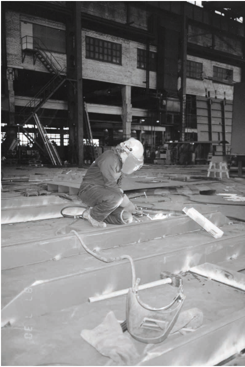
In 1987, the welder is wearing a helmet, protective mask, a dark glass in front of her eyes and safety shoes. She is equipped with hearing protection but has not deemed it necessary to wear any and appears to be wearing earplugs instead. In addition, there appears to be no ventilation from the welding fumes, which would have been employed when working in a more confined space. Rauma Maritime Museum RMM34383.
