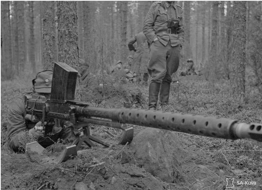
Picture 4. Famed designer Aimo Lahti's L-39 anti-tank rifle only entered widespread service in the Continuation War, when it was no longer powerful enough to penetrate the armor on Soviet tanks. SA-kuva CC BY 4.0.
