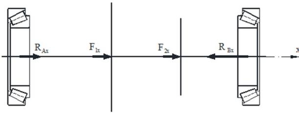
Figure 2. Calculation scheme of axial support reactions
