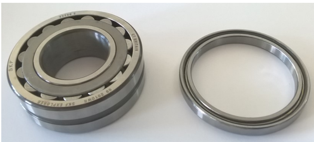
Fig. 3. The spherical roller bearing on the left and the deep groove ball bearing lubricated by grease on the right. The outer diameter of both bearings is 62 mm.
