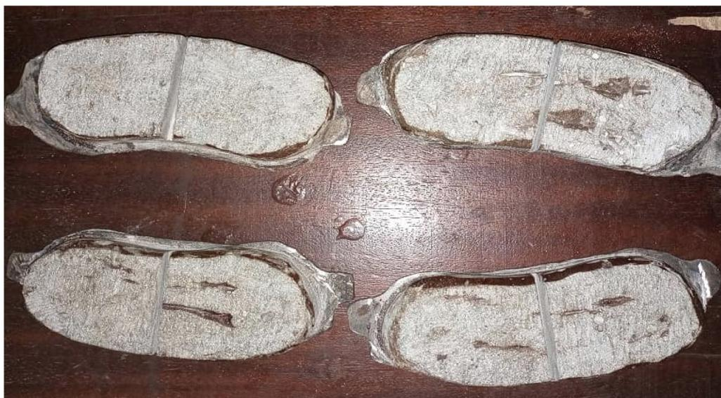
**Figure 15:** Typically finished CHR250 brakepad samples with 250 µm grains Size on backplate
